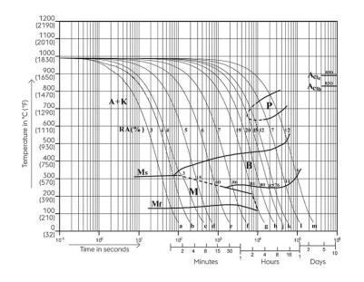
Austenitising temperature: 1025°C (1877°F) Holding time: 15 minutes 5...100 phase percentages 0.5...180 cooling parameter, i.e. duration of cooling from 800 - 500°C (1472-932°F) in s x 10<sup>-2</sup>
